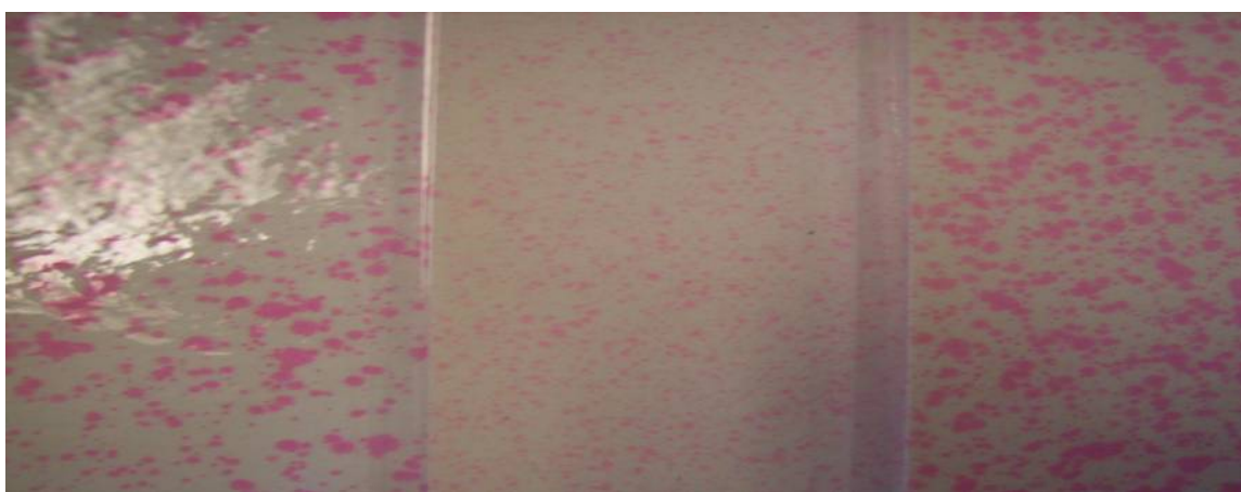
Picture 10 Different nozzle size, same water rate, giving greater coverage. (Ohio USA)
