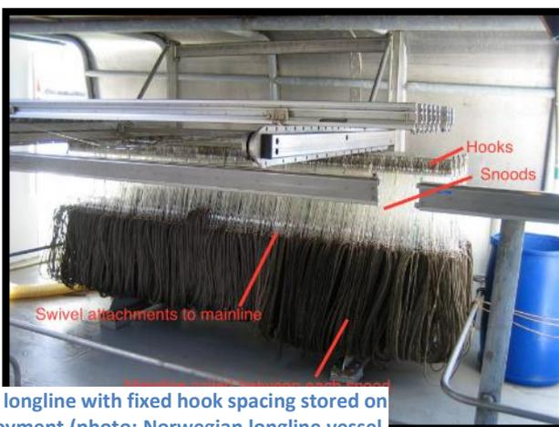
Figure 6: Automatic longline with fixed hook spacing stored on magazines for deployment (photo: Norwegian longline vessel, 31/10/2014)
